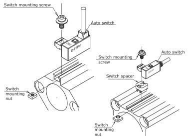
1) Slide the auto switch mounting nut inserted into the mounting rail and set it at the auto switch mounting position.
