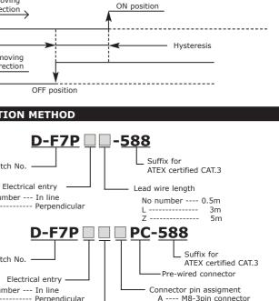
This product is a Solid State Auto Switch of direct mounting specification of the installation PNP output type. Switch should only be used in areas in which potentially explosive atmospheres are unlikely to be present or only
