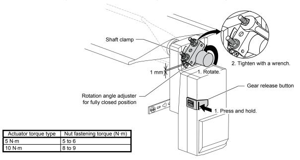
Figure 14. Complete installation of the actuator body
