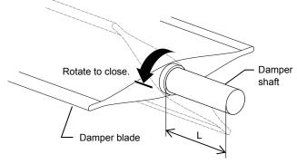
Figure 11. Damper shaft
