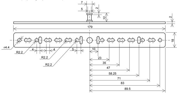
Figure 4. Dimensions: Universal bracket (mm)
