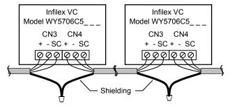
Splice the shielding with twist-on wire connectors.
