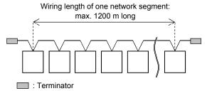
Figure 21. Wiring length of BACnet MS/TP network segment
