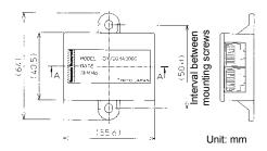
Figure 28. Modular branch unit: Part No. DY7203A0000
