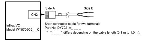
Figure 20. Connection of the connector cable for two terminals to Infilex VC
