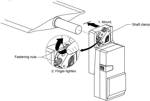
Figure 12. Temporal installation of the actuator body
