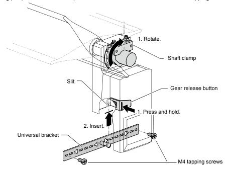
Figure 13. Attaching the universal bracket
