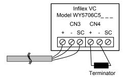
Figure 25. Terminator connection to Infilex VC
