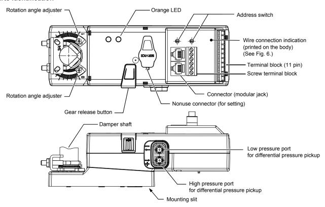
Figure 5. Parts identification
