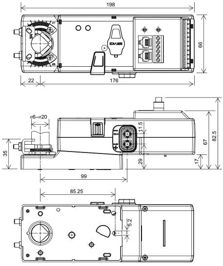
Figure 2. Dimensions: 5 N·m torque type (mm)
