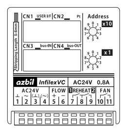
Figure 6. Wire connection indication printed on Model VY5706C5\_3\_
