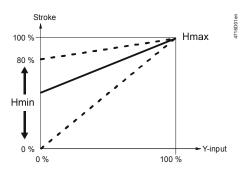
For  $k_{vs}$  reduction (DIL switch 4 in position ON), the stroke is limited to 63% mechanical stroke. 63% of full stroke then corresponds to an input/output signal of 10 V. If, in addition, the stroke is limited to 80%, for example, the minimum stroke is 0.63 x 0.8 = 0.50 of full stroke.
