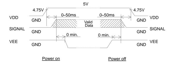
The missing pixels may occur when the LCM is driven beyond above power interface timing sequence.
