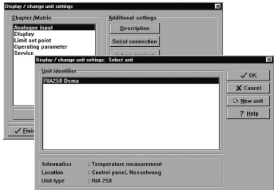
The RIA 250 can be set up extremely easily using the built-in RS 232 serial interface and the Endress+Hauser ReadWin 2000 PC software. Safe and secure set-up is made possible via on-line help text. ReadWin 2000 software and interface cable are optionally available.
